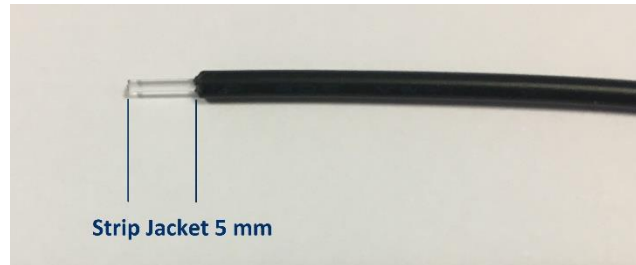
FIGURE 2. Jacket Strip Length
