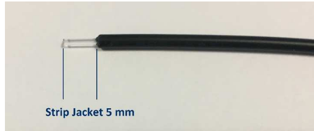
Figure 2. Jacket Strip Length
