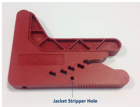
FIGURE 3. Jacket Stripper on POF cutter
