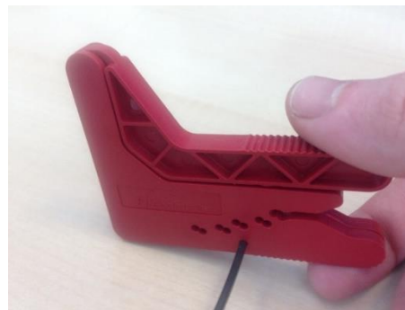
FIGURE 8. Closing of cutter
