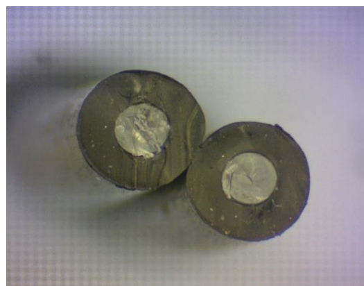
FIGURE 4. Poor quality termination finish
