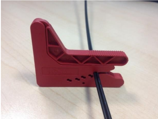
FIGURE 1. Cutting POF cable on the 'open' slot
