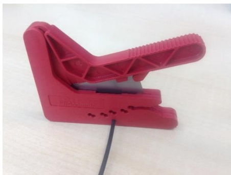
FIGURE 7. Insertion of POF cable into jacket stripper
