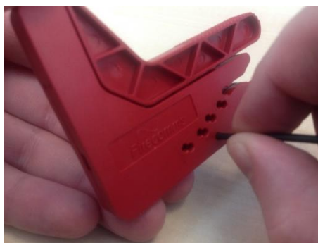
FIGURE 9. Twisting the cutter around the cable one full revolution
