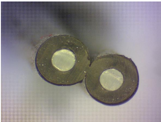
FIGURE 3. High quality termination finish
