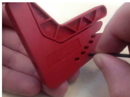
Figure 9. Twisting the cutter around the cable one full revolution
