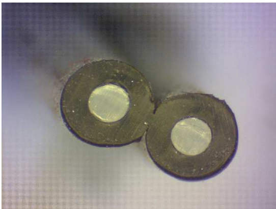
Figure 3. High quality termination finish
