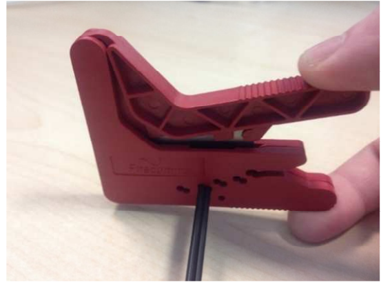
Figure 2. POF cutter in process of cutting POF cable located in one pair of 'Termination' Holes
