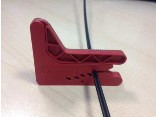
Figure 1. Cutting POF cable on the 'open' slot
