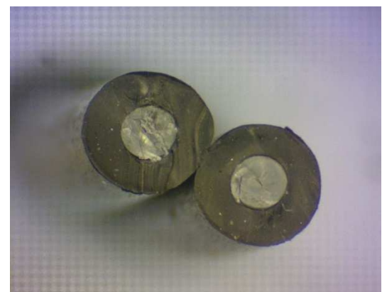
Figure 4. Poor quality termination finish
