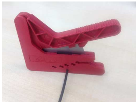
Figure 7. Insertion of POF cable into jacket stripper
