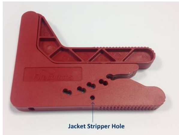
FIGURE 3. Jacket Stripper on Firecomms POF cutter
