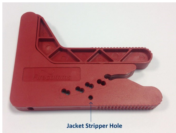
FIGURE 6. Jacket Stripper on POF cutter
