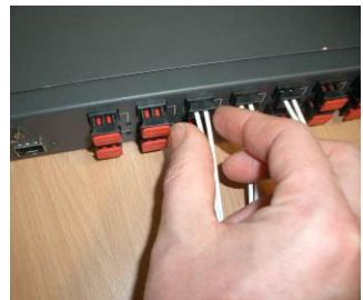
FIGURE 6 Insert both strands into OptoLock®.
