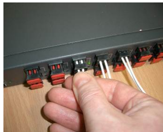
FIGURE 7 Push home to lock the clamp.
