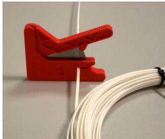
FIGURE 1 Slice the POF cable.
