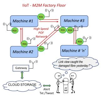
need attention, with a critical list allowing them to plan their work. As each link is tagged it is simple to identify the location of a problem link and guide staff directly to the problem. With data logging, component lifetime can be monitored and measured more accurately. This will help to bring efficiency to stocking levels for spare components.
