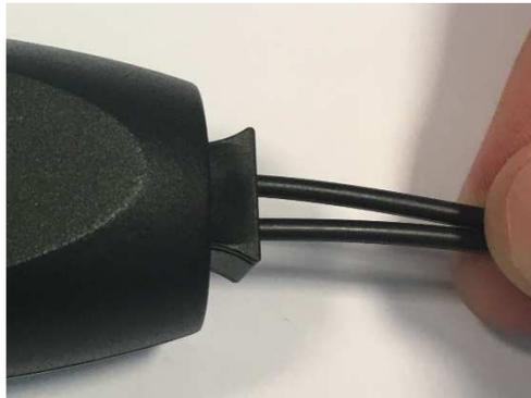
(6) Connect the CAT5 cable to both the media converter and the target equipment (e.g. a laptop, desktop, set-top-box or router).
