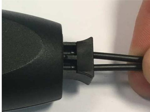
(5) Slide the fiber in until it is fully home, then press closed the OptoLock®.
