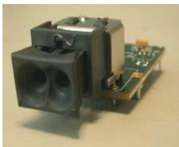
Fig. 9: Prototype gigabit POF transceiver module with an OptoLock™ bare fiber connector. Prototypes have also been constructed using a Small Media Interface (SMI) connector.
