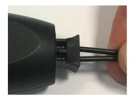
(5) Slide the fiber in until it is fully home, then press closed the OptoLock<sup>®</sup>.
